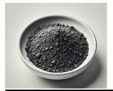
Carburizer is a Superior Carbon Additive carefully produced to enhance the Carbon content and quality of improve the production processes. It is a material which is added to molten metal to Increase its Carbon content.
