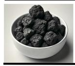
• It is a Carbon rich solid material that is used to make anodes for the Aluminium, Steel, and **Titanium** smelting industry and the feedstock for production of Synthetic Graphite
